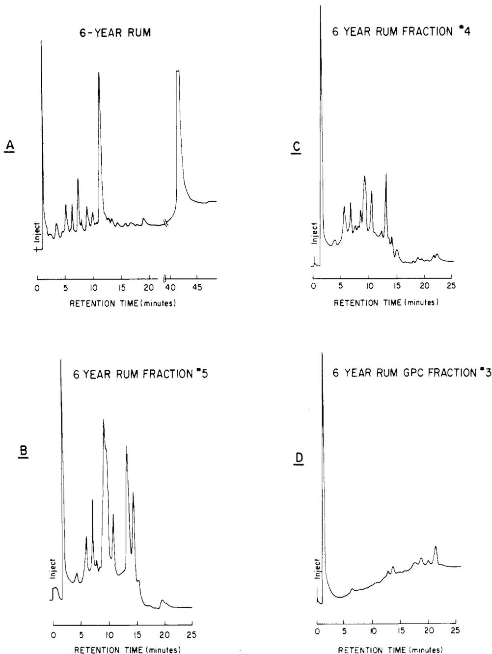
**Figure 8.** Normal partition separations of 6-year-old rum and fractions collected from preparative gpc. Operating conditions: column, 1 m  $\times$   $\frac{3}{8}$  in. i.d.; flow rate, 0.8 ml/min; solvent, chloroform; molecular weight range, 85–1000.
