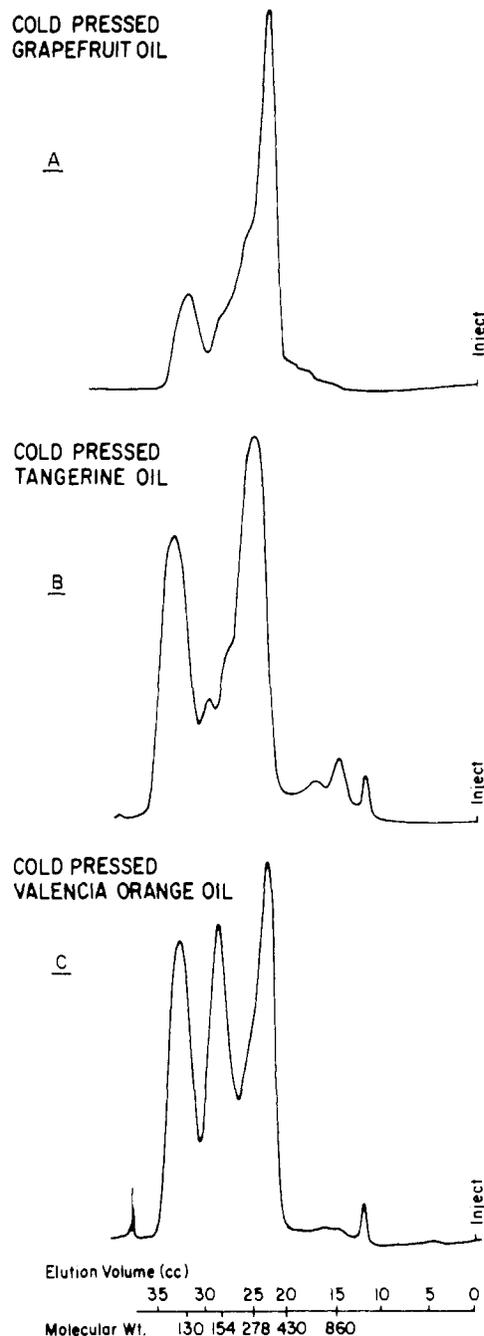
Figure 2. Steric exclusion separations of cold-pressed citrus oils. Operating conditions: column, 1 m  $\times$   $\frac{3}{8}$  in. i.d.; flow rate, 0.8 ml/min; solvent, chloroform; molecular weight range, 85-1000.
