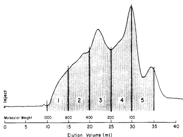
Figure 7. Preparative gpc separation of 6-year-old rum fraction. Fraction numbers are marked on the bottom of the chromatogram. Operating conditions: column, 1 m  $\times$   $\frac{3}{8}$  in. i.d.; flow rate, 0.8 ml/min; solvent, chloroform; molecular weight range, 85-1000.
