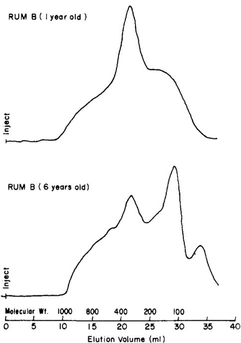
Figure 5. Comparison of 1-year-old rum and 6-year-old rum from the same distillery. Operating conditions: column, 1 m  $\times$   $\frac{3}{8}$  in. i.d.; flow rate, 0.8 ml/min; solvent, chloroform; molecular weight range, 85-1000.
