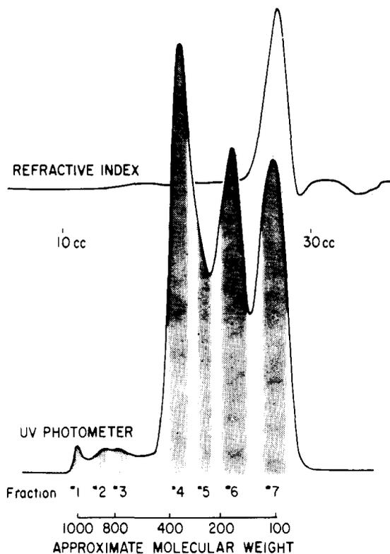
Figure 4. Fractions collected from preparative gpc for characterization by liquid chromatography. Operating conditions: column, 1 m  $\times$   $\frac{3}{8}$  in. i.d.; flow rate, 0.8 ml/min; solvent, chloroform; molecular weight range, 85-1000.
