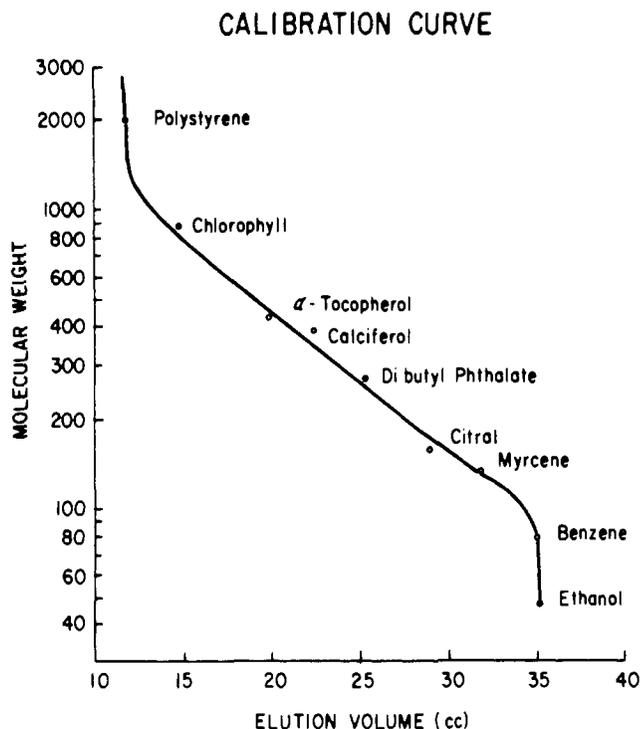
Figure 1. Calibration curve for Biobeads SX-2. Operating conditions: column, 1 m  $\times$   $\frac{3}{8}$  in. i.d.; flow rate, 0.8 ml/min; solvent, chloroform; molecular weight range, 85-1000.
