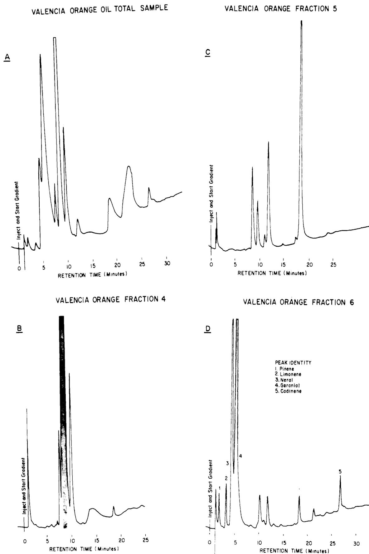
**Figure 3.** Reversed-phase liquid chromatographic separations of the total cold-pressed oil and collected fractions. Operating conditions: column, 1 m  $\times$  2.1 mm; Permaphase ODS mobile phase, linear gradient from 5% MeOH/95% H<sub>2</sub>O to 100% MeOH at 3%/min; column temp, 50°; flow rate, 1.5 ml/min; detector, uv photometer.
